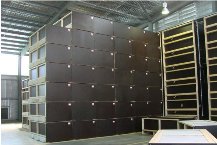
Figure 4: seed drying boxes against a vented wall (at Bejo Zaden B.V.)
