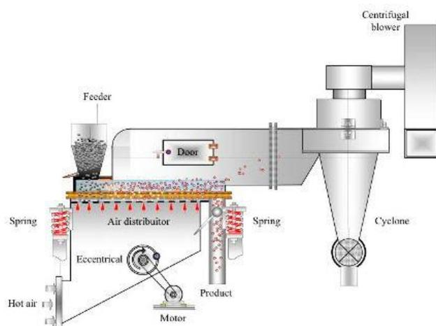
Figure 5: vibrating fluid bed seed dryer (from KTH)
