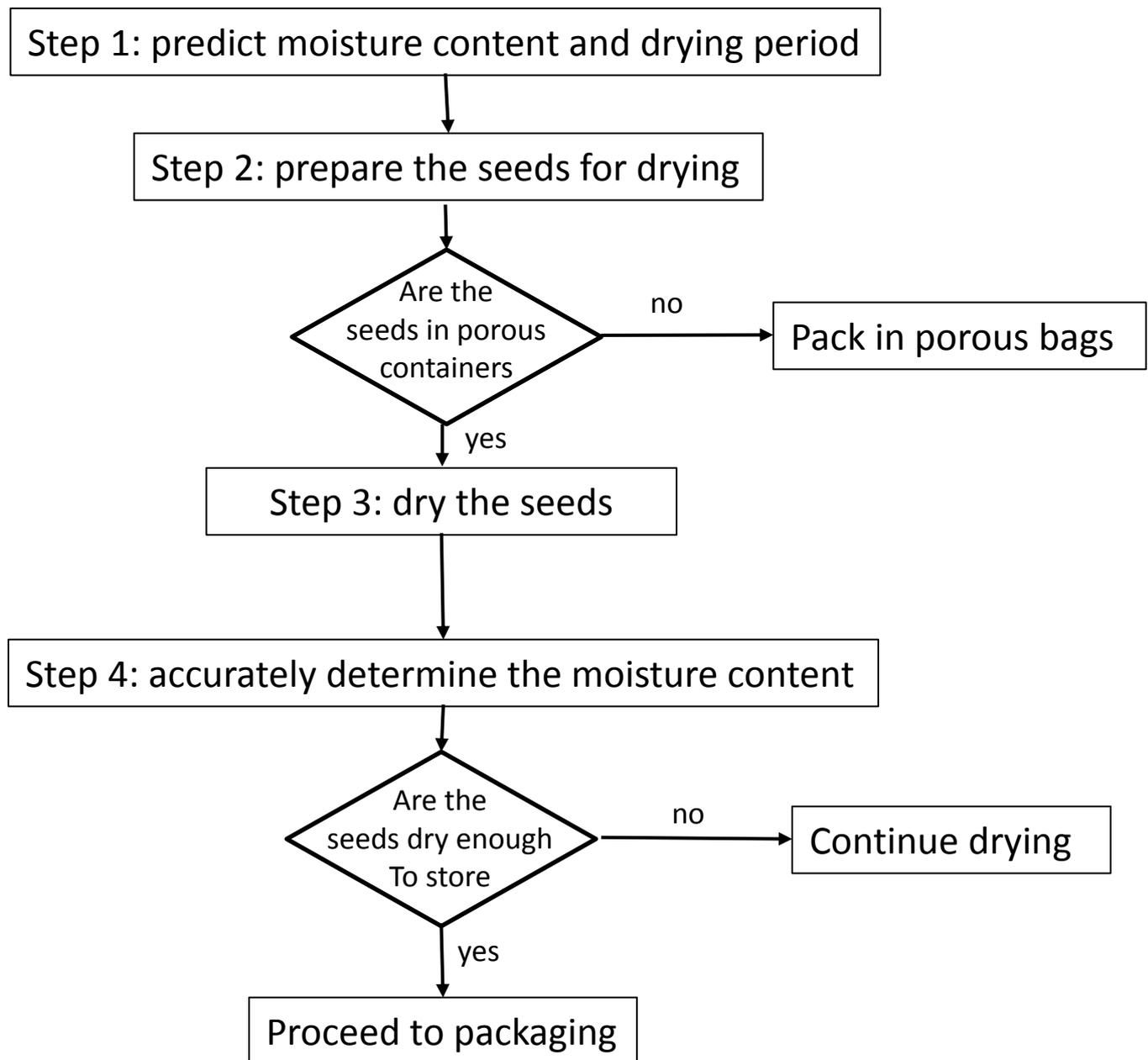
Figure 1: Seed drying procedure
