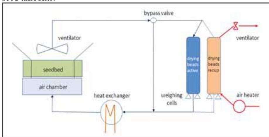
Figure 6: scheme of an indirect zeolite based seed dryer (from Centor Group)
