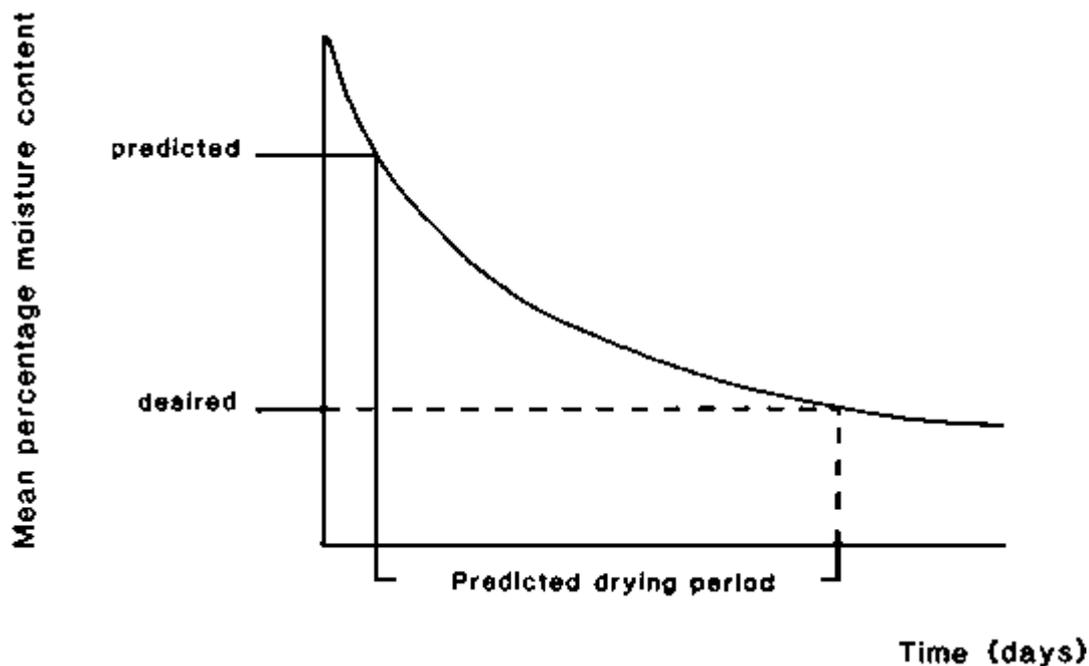
Figure 2: Typical seed drying curve
